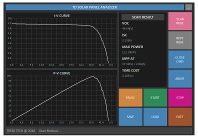
Fig.5 The I-V curve and P-V curve are plotted.
