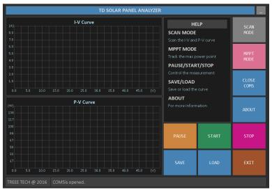
Fig.4 PC software interface after connecting to PC
